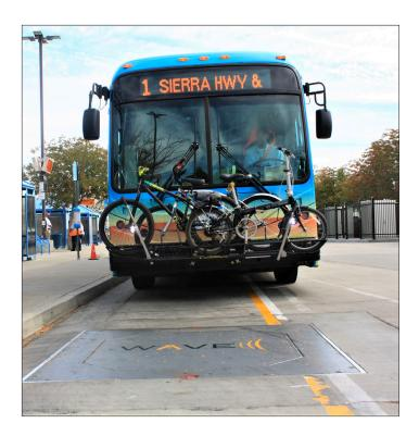
By December 2020, AVTA's fully-electric, 65-bus, local fixed-route fleet logged its four millionth mile, less than seven years after its first electric bus went into service.<sup>1</sup> Moreover, the agency covered its longest routes with a single electric bus without making changes to its schedules or vehicle count. This was accomplished because of AVTA's decision to use wireless, high-power, in-route charging from WAVE.
